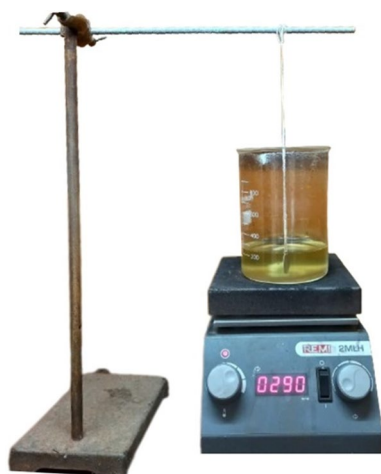
Fig. 6 Experimental setup for the spontaneous deposition of ^{210}\text{Po} on a silver disc
