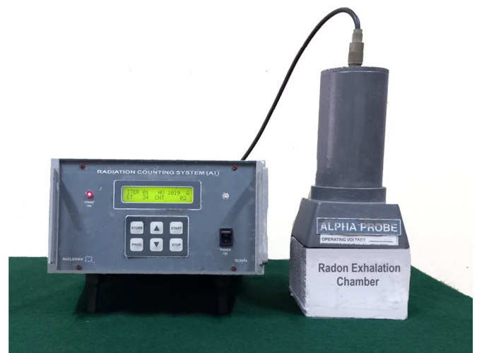
Fig.3. Measurement of 222 Rn exhalation rate from soil samples using alpha counting system.
