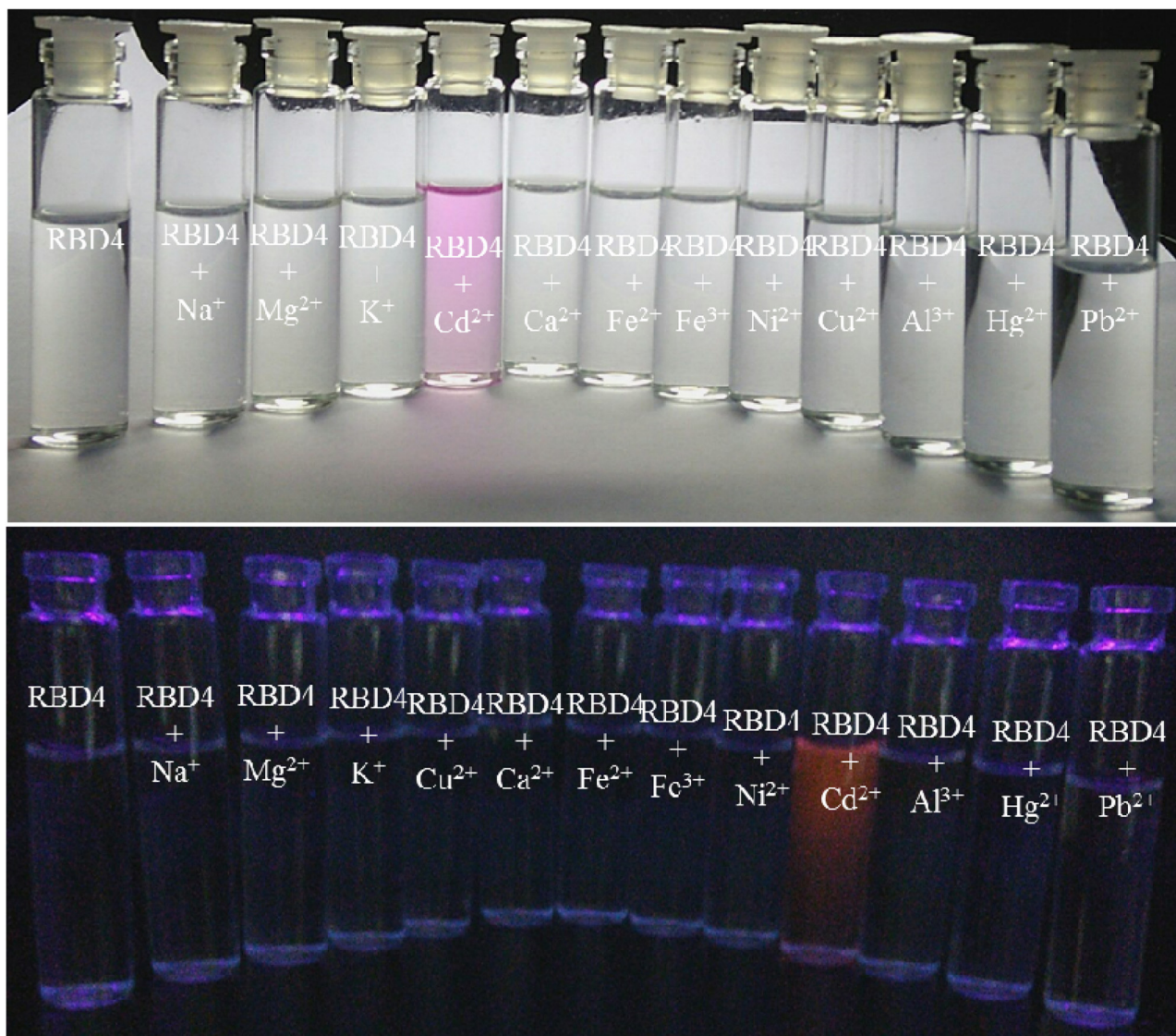
Fig. 4. Visual color change of probe RBD4 (100 μM) upon the addition of various metal ions (2 equivalents) in ACN/HEPES buffer (2:8, v/v, 10 mM, pH 7.2) (Top). Fluorescence color change of probe RBD4 (100 μM) upon the addition of various metal ions (2 equivalents) in ACN/HEPES buffer (2:8, v/v, 10 mM, pH 7.2) (Bottom).
